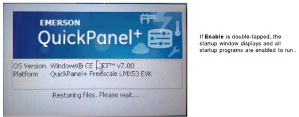
Figure 17: Start-Up Window following Enable
