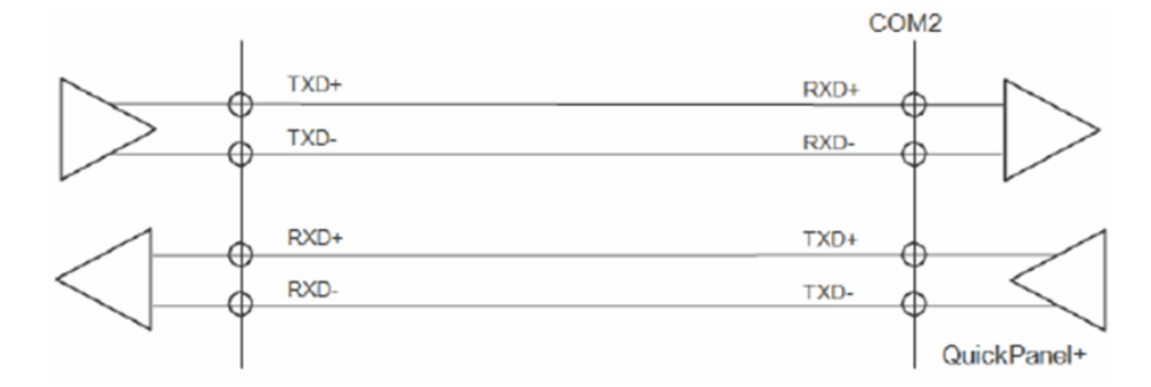
Figure 77: Example of Full-Duplex (RS-422 Mode) Connection
